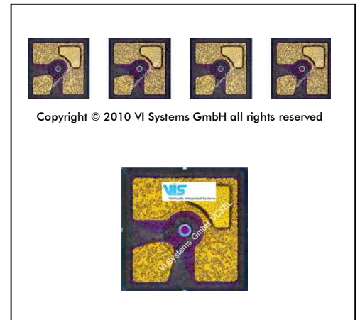
Microscope images of a 1x4 VCSEL array chip and a single VCSEL die. The actual products may vary in appearance and size.
