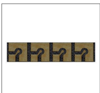
Ultrahigh-Speed VCSEL Array (28 Gbit/s) V25-850C4 / V25-850C12
